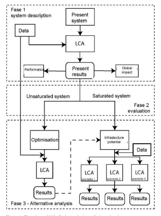
Figure 1. Flowchart of Life Cycle Analysis applied to a local transport system.
